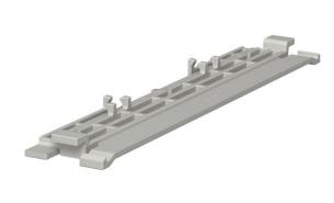
Cover clip for better and easier laying of lines in the WDK trunking. The cover fixing device can be moved along the entire length of the trunking. The cover clip is locked on one side and moved forward. This provides a 30° opening, meaning that cable routing is very simple. From trunking widths of 110 mm, the cover clips can also be used as a mounting aid
